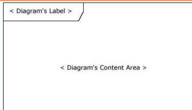
Figure 1: An empty UML 2 frame element
